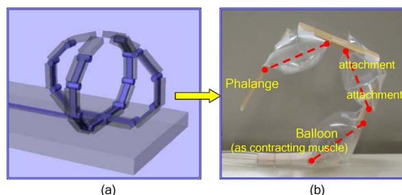
FIG. 1. Schematic drawing of a microhand device with four fingers articulated by balloon joints, mimicking the flexion and extension capabilities of the human hand in microscale. (b) The actuation mechanism is illustrated in a simplified centimeter-scale experiment, in which the inflating of the balloons (plastic bags) shortens the distance between the attachment points, drawing up the Plexiglas phalanges.
