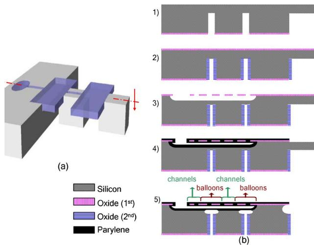
FIG. 2. Microhand fabrication process. (a) shows a three-dimensional schematic of one finger. For simplicity, only two phalanges and two balloon joints are shown. (b) illustrates the process flow in the cross section of (a).
