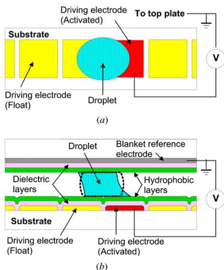
**Figure 1.** Popular two-plate configuration EWOD chip with asymmetric electrode arrangement. Once voltage is applied, the change in the meniscus shape (from the dotted shape) caused by contact angle changes induces a gradient inside the droplet. (a) Top view; (b) cross-section view.
