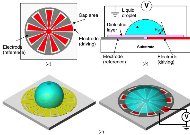
**Figure 3.** EWOD of a sessile drop on single-side coplanar electrodes: (a) electrode arrangement (top view); (b) cross-section view with voltage applied; (c) contact angle change on coplanar electrodes.
