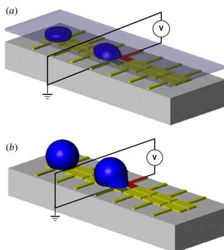
**Figure 7.** Droplet movement by EWOD on single-side coplanar electrodes, each unit consisting of two sub-electrodes in this figure: (a) with top cover plate (i.e., droplet squeezed to a disk shape); and (b) with no cover plate (i.e., droplet formed to a spherical shape).
