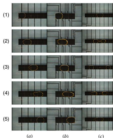
**Figure 8.** Transportation of a droplet by EWOD on coplanar electrodes under parallel-plate configuration: (a) transportation on two-sub-electrode pads; (b) transportation on six-sub-electrode pads; (c) cutting and merging of a droplet on two-sub-electrode pads.
