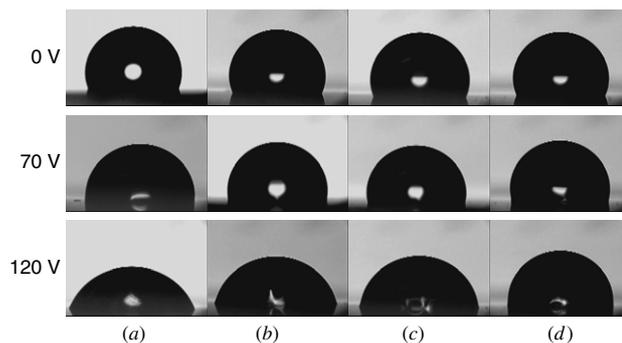
**Figure 5.** Contact angles of sessile drops on coplanar electrodes of figure 3 for four different gap areas under EWOD actuation. (a) 2% gap area, (b) 20% gap area, (c) 40% gap area, (d) 60% gap area.
