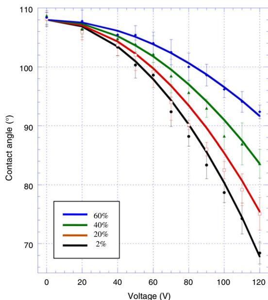
**Figure 6.** Contact angle changes for EWOD on coplanar electrodes with 2%, 20%, 40% and 60% gap areas. Theoretical values (by equation (3)) are plotted with solid lines while actual data are plotted with geometric dots with error bars ( $\pm\sigma$ ). The data from chips with 10% gap area were also consistent but not plotted in this graph for the readability of data.
