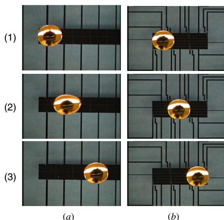
**Figure 9.** Manipulation of a droplet by EWOD on single-side coplanar electrodes on the open surface (i.e., no cover plate). The droplet volume is  $\sim 2 \mu\text{l}$ , which is  $\sim 20$  times that of figure 8. (a) Transportation on two-sub-electrode pads; (b) transportation on six-sub-electrode pads.
