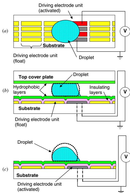
**Figure 4.** Droplet moving by EWOD on coplanar electrodes. (a) Top view showing driving electrode units, each consisting of sub-electrodes (four in this figure). (b) Driving in parallel-plate configuration with the top plate having no electrode. (c) Driving in open-plate configuration (i.e., no cover plate). Note the initial shapes of droplets before contact angle changes for the two cases, drawn with broken lines.
