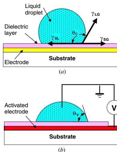
**Figure 2.** Contact angle changes by electrical potential on the EWOD surface: (a) initial state; (b) activated state.
