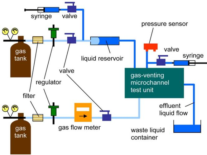
Fig. 6. Experimental apparatus to test the gas-venting microchannels made with porous hydrophobic membranes.
