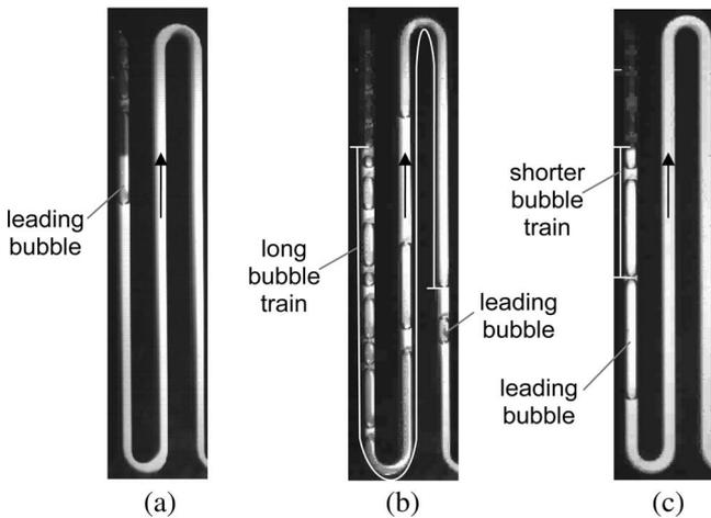
Fig. 8. Venting threshold. (a) Water:  $P_l - P_o = 5.5$  kPa. (b) 10-M methanol:  $P_l - P_o = 5.5$  kPa. (c) 10-M methanol:  $P_l - P_o = 3.4$  kPa.
