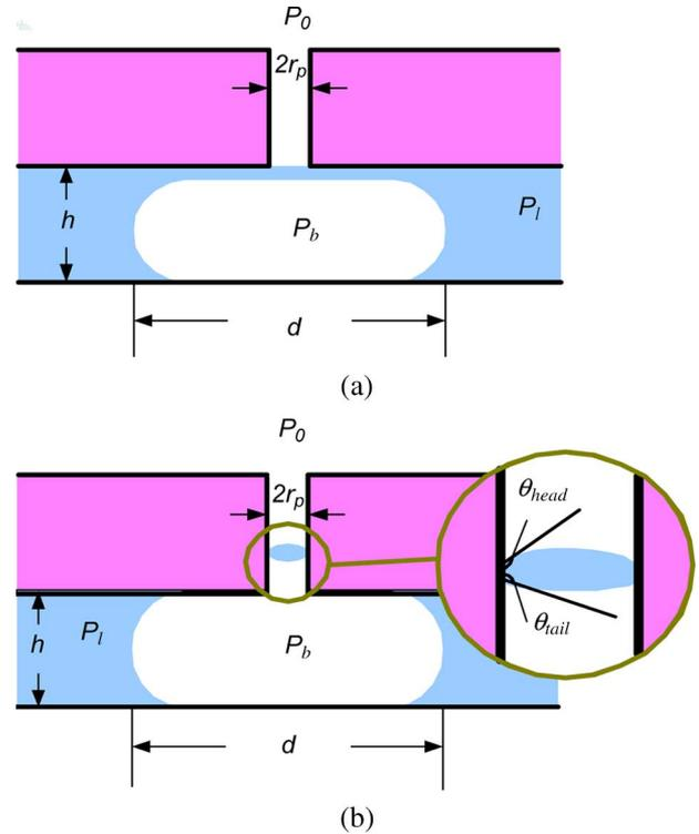
Fig. 9. Hypothetical explanations for the venting threshold: (a) by a thin liquid film and (b) by a trapped droplet.
