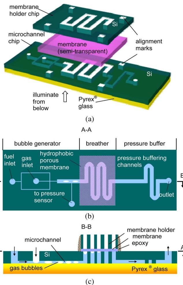
Fig. 5. Gas-venting microchannel with on-chip bubble injector. (a) Perspective view during alignment and bonding. (b) Horizontal cross section (A-A view) of a completed device. (c) Vertical cross section (B-B view) of a completed device.
