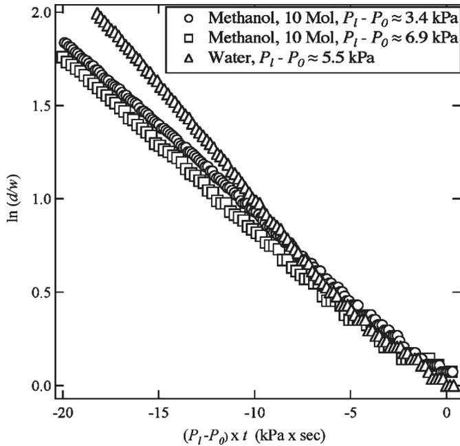
Fig. 10. Evolution of elongated bubble length  $d$  as a function of time and transmembrane pressure (experimental data obtained in a gas-venting microchannel constructed by the porous polypropylene membrane).
