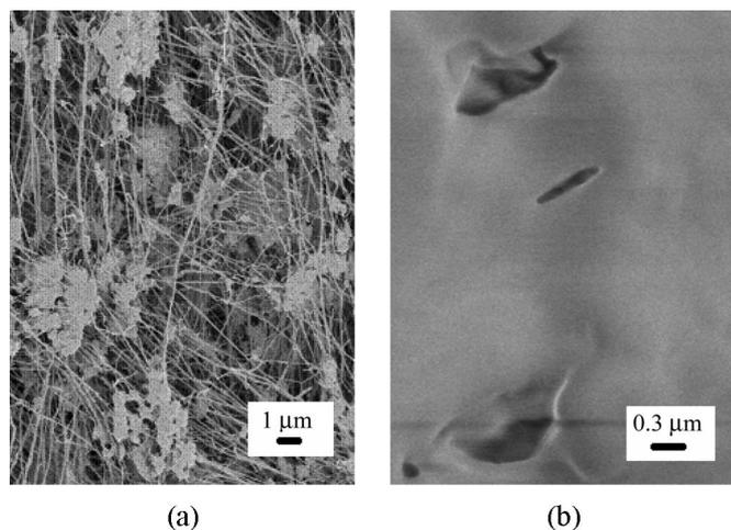
Fig. 4. SEM pictures of the porous membranes' surface. (a) Porous PTFE. (b) Porous polypropylene.
