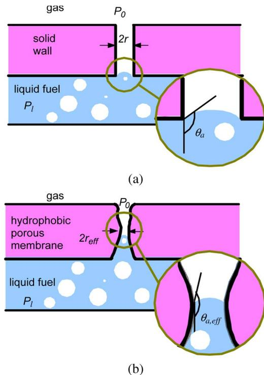
Fig. 2. Small meniscus in a hydrophobic capillary prevents liquid leakage. (a) Idealized straight and smooth capillary. (b) Realistic capillary of irregular shape.
