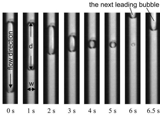
Fig. 7. Exemplary venting process in a gas-venting microchannel. The video clips were taken from a two-phase flow of 10-M methanol and nitrogen gas bubbles along a microchannel made with porous polypropylene membrane. The device is horizontally positioned with respect to gravity.
