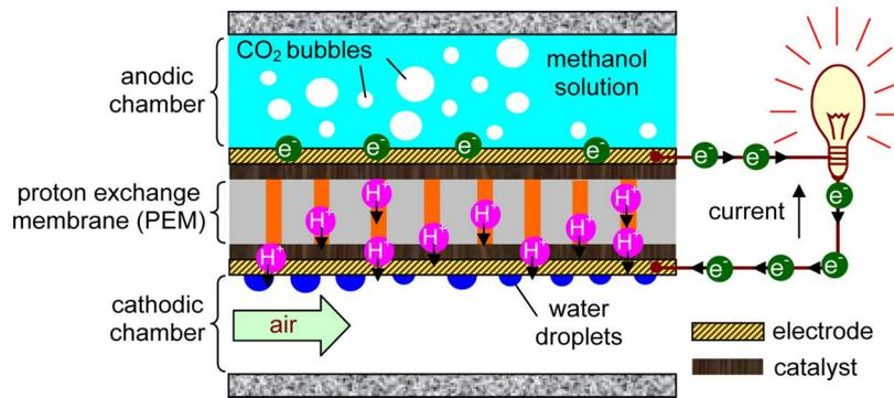
Fig. 1. Working principle of a DMFC.
