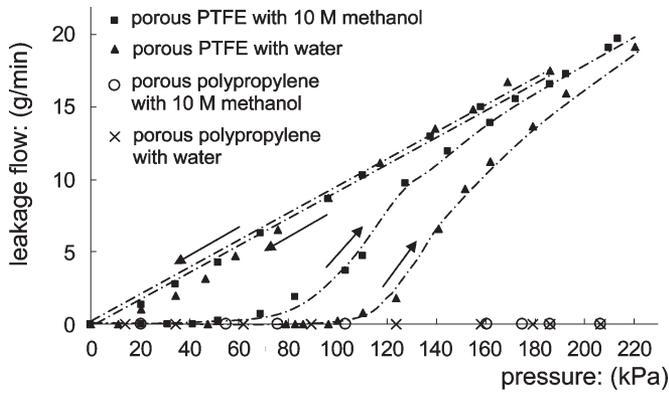
Fig. 3. Flow–pressure curve of hydrophobic nanoporous membranes for water and 10-M methanol.
