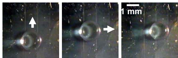
Figure 9. A sequence of pictures showing a translational droplet between two superhydrophobic surfaces (at 24 V_{rms} , 10 Hz).
