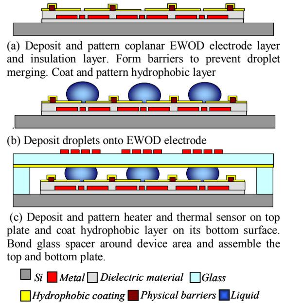
Figure 6: Process flow for EWOD-driven thermal switch testing device.
