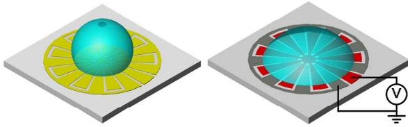
Figure 2: A water sessile droplet switching between beading and wetting on the EWOD device with coplanar electrodes [6].
