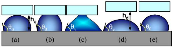
Figure 3: Hysteresis in droplet attachment-detachment. (a) EWOD off. About to touch top plate at height  $h_a$ . (b) Bridge formed. (c) EWOD on. Spreads on bottom but still bridged. (d) Detaches by elevating top to  $h_d$ . (e) EWOD off to make droplet tall but cannot connect. Need to lower top to  $h_a$  to touch it again.
