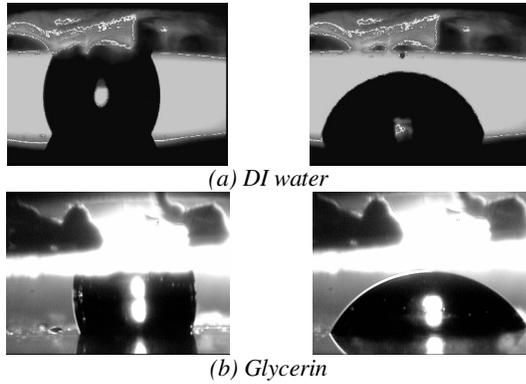
Figure 5: Droplets switch on/off on coplanar EWOD device with 4000Å  $Si_3N_4$  and 2000Å Teflon driven with 1 kHz 70  $V_{pp}$ . The gap between top and bottom plates is approximately 1 mm.
