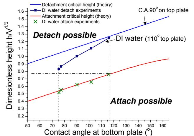
Figure 4: Static experiment for droplet detachment and attachment.
