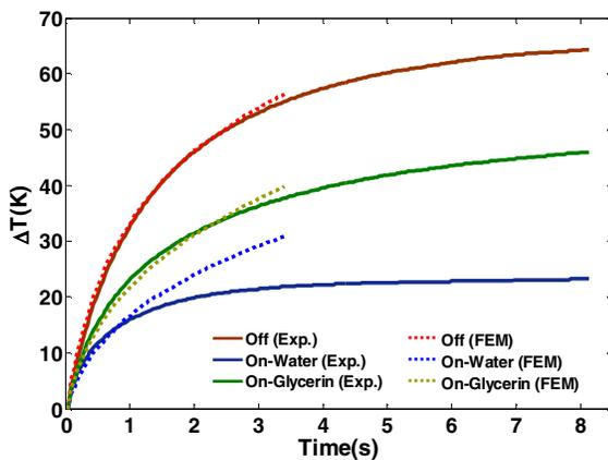
Figure 8: Measured temperatures change by switch on and off using water and glycerin. FEM results for comparison.
