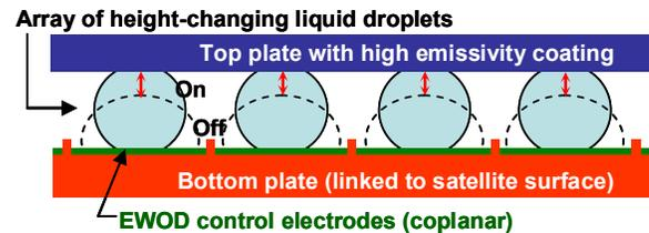
Figure 1: Conceptual design of the proposed EWOD-based thermal switch configured as a variable emittance radiator.
