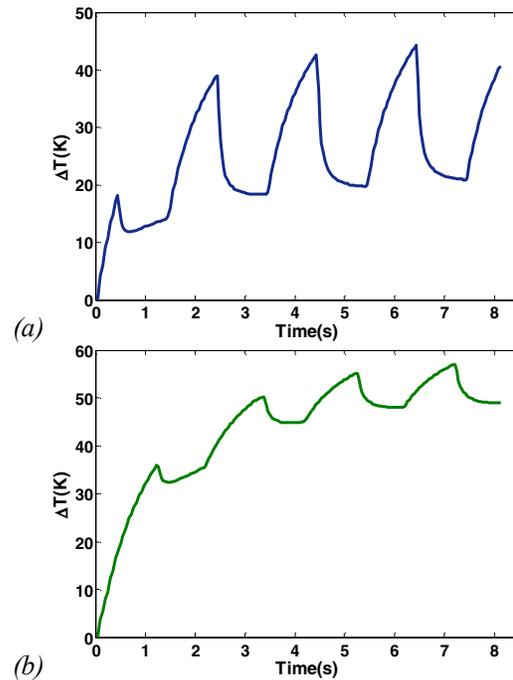
Figure 9: Experiment data of 1 Hz thermal switching test using (a) water and (b) glycerin droplets.
