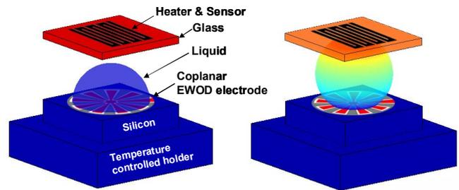
Figure 7: Schematic experimental setup, Thermal switch off (left) and switch on (right). At test, top is heated to simulate satellite surface and its temperature measured, while bottom is at constant temperature.
