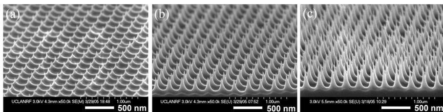
Figure 2. Scanning electron microscopy images of sharp-tip nanopost structures: (a) Nanopost-Low; (b) Nanopost-Mid; (c) Nanopost-High.
