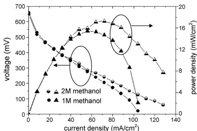
Fig. 4. Characterization of the MEA used for the  $\mu$ DMFC. The tests were performed under room temperature with  $3 \text{ mL min}^{-1}$  methanol flow at anode and  $\sim 100 \text{ mL min}^{-1}$  oxygen flow at cathode.
