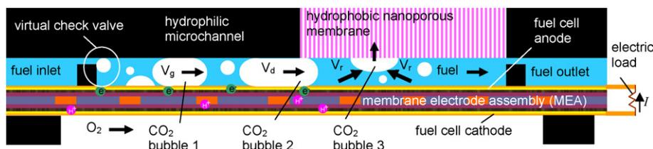
**Fig. 2.** Schematic description of the embedded self-circulation of liquid fuel by intrinsic  $\text{CO}_2$  gas bubbles.
