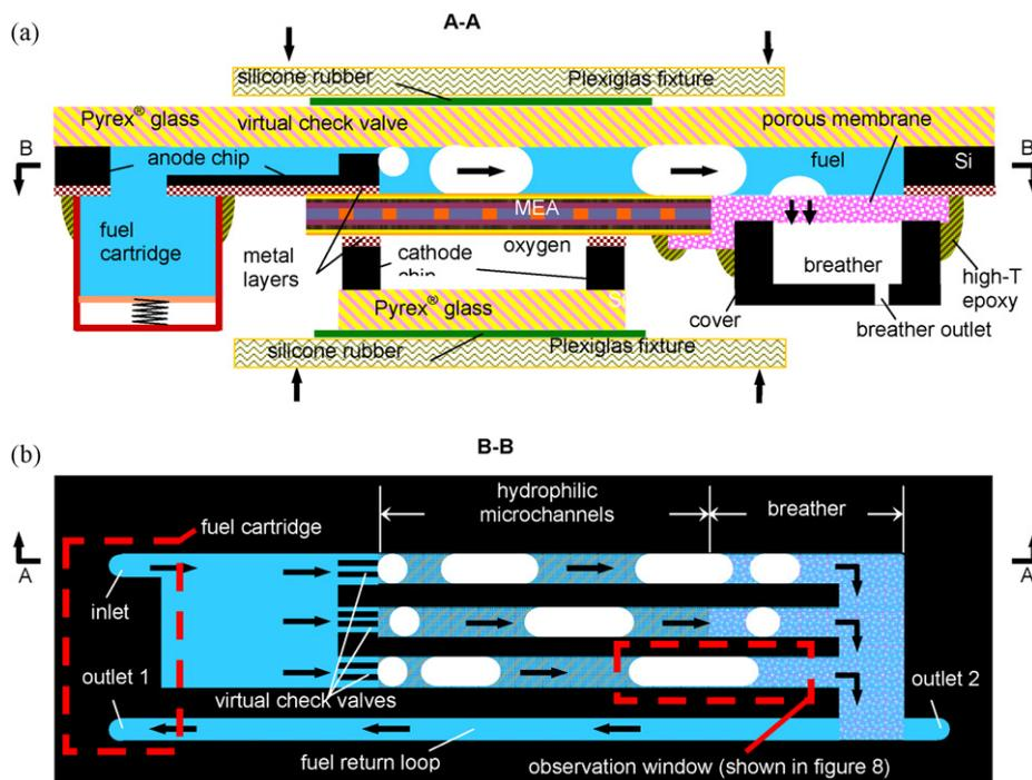
Fig. 3. Schematic drawings of the assembled self-circulating  $\mu\text{DMFC}$  device. (a) Cross-sectional view (A–A plane of the top view); (b) top view (B–B plane of the cross-sectional view).
