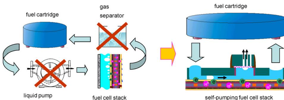
**Fig. 1.** It is proposed that the anode configuration can be greatly simplified for miniature fuel cells (e.g.,  $\mu$ DMFC) by eliminating gas separator and liquid pump from the conventional configuration (shown left) and integrating the functionalities into an embedded self-circulation structure (shown right). The self-circulation mechanism has so far been proven by providing gas bubbles extrinsically through electrolysis and injection in a controlled manner [19].
