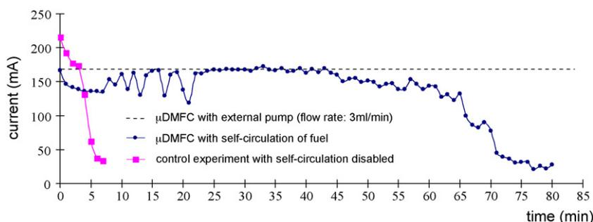
Fig. 5. Self-circulation mechanism is verified by measuring the current output of a given  $\mu$ DMFC device under three different scenarios for fuel delivery. The device operated over 70 min with the self-circulation of fuel, while it lasted less than 5 min with the self-circulation disabled (i.e., under passive operation). The device operation with an external fuel pump delivering an unlimited amount of fuel is shown as a top reference.
