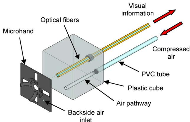
Fig. 7. Illustration of the packaging scheme. Plastic cube with holes for an air pathway and optical fibers is bonded to the back of the microhand chip. The optical fiber bundle is exposed to the front side through the palm opening after packaging. The air pathway is aligned to meet the air inlet at the backside of the microhand chip.
