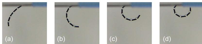
Fig. 10. Side view of a single finger that is 4 mm in length, when (a) no pressure is applied, (b) 140 kPa, (c) 280 kPa, and (d) 410 kPa is applied (0, 20, 40, and 60 lbf/in<sup>2</sup> equivalent, respectively).
