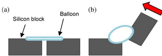
Fig. 1. Schematic illustration of the balloon actuator. (a) Balloon connects two silicon blocks. (b) When the balloon inflates with compressed air, the attached blocks make a relative out-of-plane motion against each other due to the tension of the balloon.
