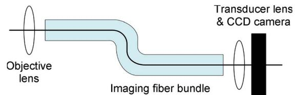
Fig. 4. Schematic of optical system used in this paper. The system consists of the following: 1) an objective lens; 2) an imaging bundle; and 3) a bundle-camera transducer lens and CCD camera.
