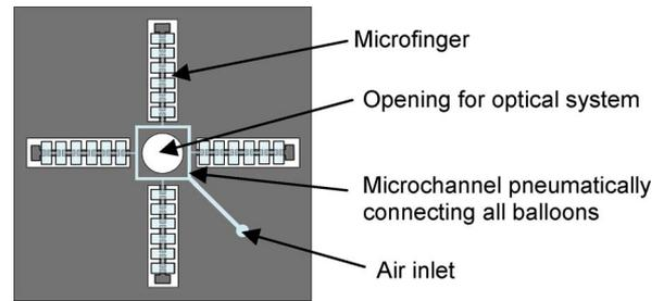
Fig. 3. Four-finger microhand design with a 1.5-mm opening in the "palm." Each finger is 4 mm in length, and the hand forms a fist of 5 mm in diameter at 240 kPa. The distance between the opposing fingers at the anchors is 2.6 mm, and all the balloons are pneumatically connected by microchannels and to the air inlet.
