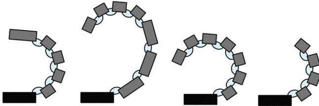
Fig. 2. Various finger curling shapes are determined by the number of joints and the varying lengths of phalanges.
