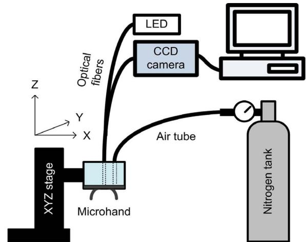
Fig. 9. Schematic of the experimental setup. A pressure-regulator-controlled nitrogen tank and CCD camera are connected to the microhand package by a PVC tube and optical fibers, respectively. Real-time images sent from the palm of the microhand are transferred via optical fibers to the CCD camera that shows the images to an operator. The microhand is held by an XYZ stage that controls the movement.
