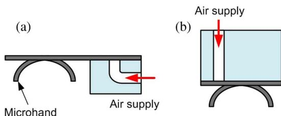
Fig. 6. (a) Air inlet in the frontside of the microhand chip. Previous microhands [10], [22] had the air inlet in the frontside, limiting the operation of the microhand due to the thick packaging attached in the same direction as the microhand’s finger motion. (b) Newly developed microhand with the air inlet located in the back of the microhand chip. Because the packaging is attached in the back, the microhand can move and be operated without any obstruction by the packaging.
