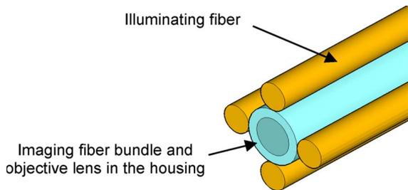
Fig. 5. Arrangement of illuminating fibers and the imaging fiber bundle sealed with the objective lens in the housing. Four illuminating fibers (250  $\mu\text{m}$  in diameter each) are surrounding the imaging fiber housed with the lens with 550- $\mu\text{m}$  overall diameter.
