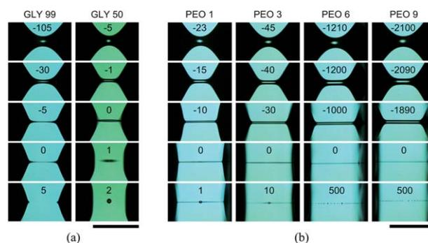
**Fig. 5** (a) High-speed video frames of viscous (GLY 99) and inertial (GLY 50) breakup of aqueous glycerol solutions. Frame zero is assigned to the frame before the filament disappears. (b) High-speed video frames of elastic breakup of aqueous glycerol + PEO solutions. Frame zero is assigned to the frame before beads-on-a-string form along the filament. For both (a) and (b), frames were captured at a rate of 30 000 fps. The scale bars are 0.5 mm. See videos of GLY 50 and PEO 9 in the ESI†.
