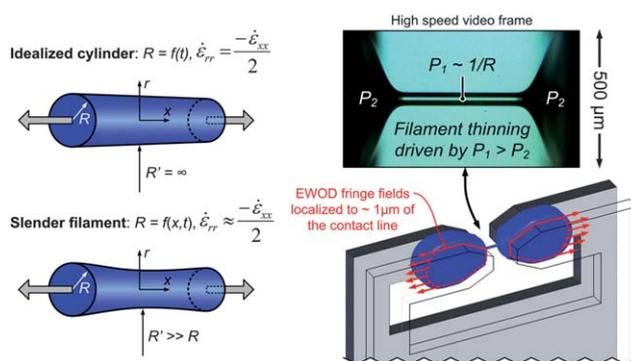
**Fig. 4** Left: illustrations of idealized and realistic filament shape. Right: a high-speed video frame showing a measured PEO 9 filament, and a 3-dimensional schematic of the rheometer chip with red lines indicating the location of EWOD fringe fields.
