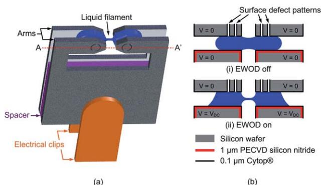
**Fig. 1** (a) Three-dimensional sketch of a loaded chip and close-up of the liquid bridge. (b) Cross-sections A–A' of (a).
