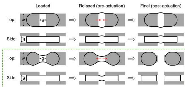
**Fig. 2** Illustrations summarizing observations of partially wetting liquid samples loaded onto straight (top) and tapered (green dashed box) chip arms.
