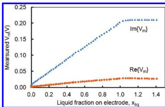
**Figure 4.** Experimental relationship between MeCN liquid fraction  $x_{liq}$  and measured signal  $V_m$ . Real and imaginary components of the measured voltage are shown.
