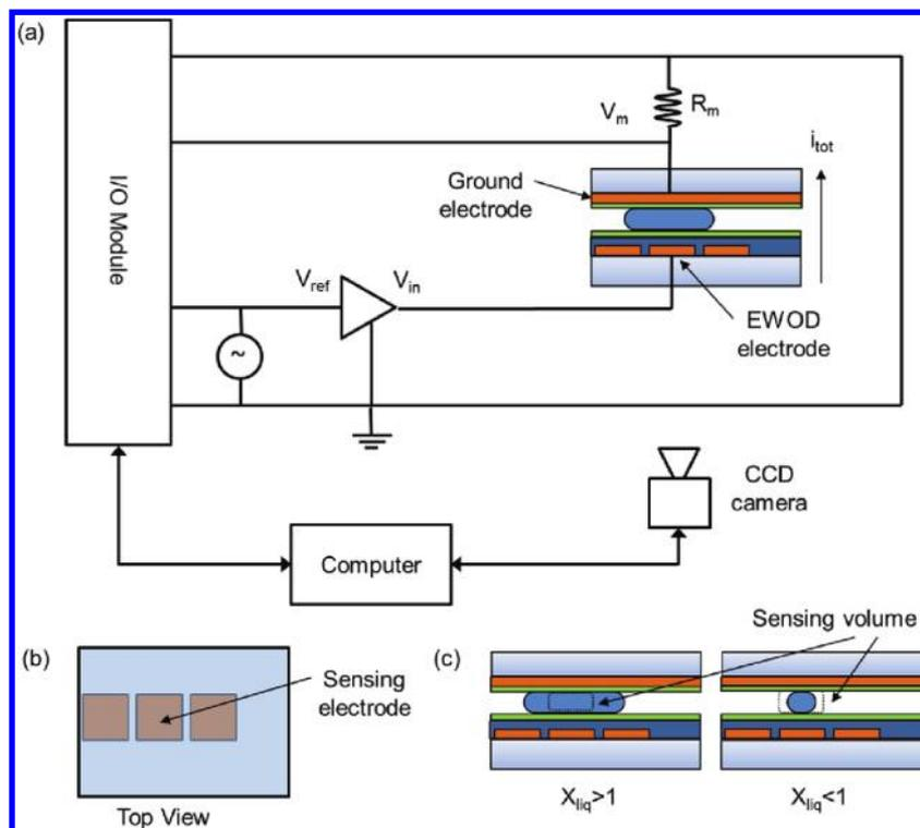
**Figure 2.** Schematic of the liquid detection system. (a) Diagram of the impedance measurement system. (b) Top view of the EWOD chip. (c) Side view of the chip showing sensing volume for the cases where droplet is larger than the electrode ( $x_{liq} > 1$ ) or smaller than the electrode ( $x_{liq} < 1$ ).
