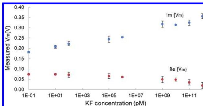
**Figure 6.** Measured signal  $V_m$  with 100 V<sub>rms</sub> excitation potential at 10 kHz, for different concentrations of potassium fluoride (KF) in water. Due to the change in resistivity and permittivity from the dissolved KF, the liquid impedance changes, leading to a change in the total device current, as measured by the change in both real (red) and imaginary (blue) components of the measured signal.
