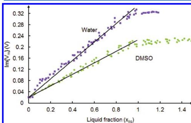
**Figure 5.** Relationship between  $\text{Im}\{V_m\}$  and droplet size ( $x_{liq}$ ) for water and DMSO.
