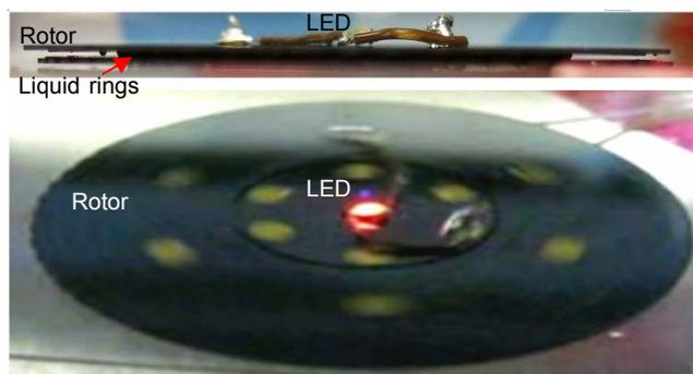
Figure 7: A red LED blinking at the center of a rotor (no stator in this device) that is being rotated by blowing air.
