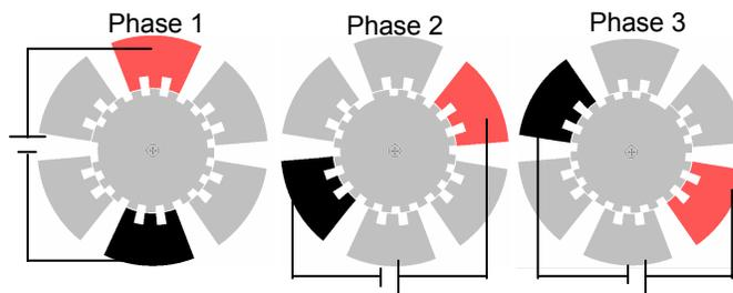
Figure 6: Three-phase electrostatic actuation.
