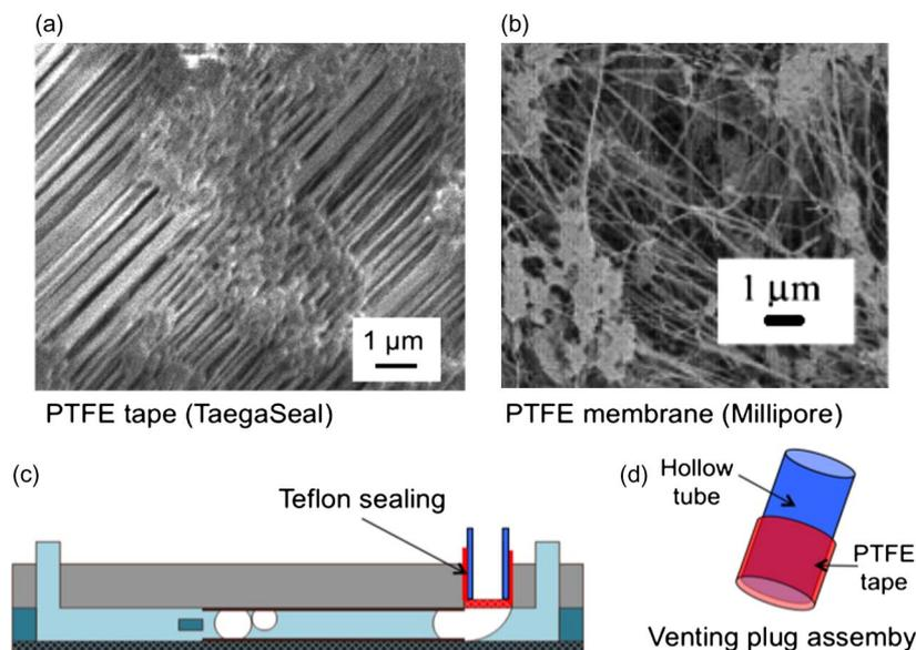
Fig. 3. (a) SEM of PTFE tape (TaegaSeal) and (b) PTFE membrane (Millipore). Although PTFE tape has more directional pore patterns, they both have pore sizes in the order of 100 nm. (c) In the final device, venting plug assembly is plugged into the venting hole. PTFE tape wrapped around a hollow tube gives air-tight sealing, and (d) hollow tube of venting plug assembly gives a structural support to the PTFE venting membrane.
