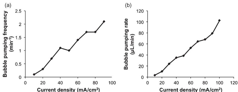
Fig. 6. Pumping frequency and rate of designed fuel cell. (a) Frequency of bubble pumping generally increases with the current density generated. Since the frequency only counts the number of bubbles, it does not directly account for the volume of pumping. (b) Measured with the volume of each bubble leaving the venting site, the bubble pumping rate is found proportional to the current density.
