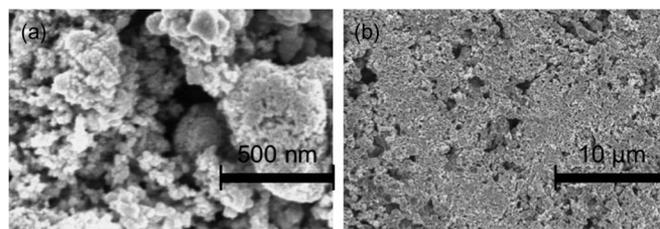
Fig. 9. SEM images of solution-deposited Pd electrocatalyst. (a) At closer view, Pd black has cluster-like structures with nanometer scale roughness. (b) In micrometer scale view, the catalyst layer is rather flat and lacks the hierarchical structure of (a).
