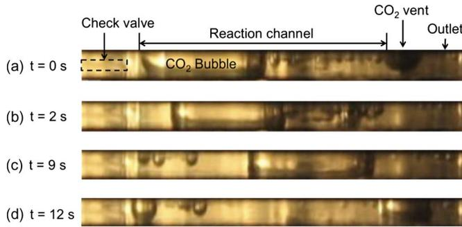
Fig. 5. Snapshots of bubble pumping taken during fuel-cell operation. 1 M formic acid was used as fuel mixed in 1M sulfuric acid under ambient pressure and room temperature.  $\text{CO}_2$  bubbles successfully nucleated, grew, merged, moved along the diverging channel, and vented out of the channel through the hydrophobic nanoporous membrane.
