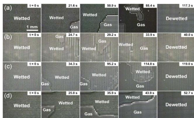
Fig. 6. Dewetting by electrolysis of microposts with a pitch of  $100\ \mu\text{m}$  and gas fractions of (a) 85%, (b) 90%, (c) 95%, and (d) 98%.
