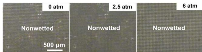
Fig. 10. Developed SHPo surface remained nonwet in water of an increasingly high pressure, when the voltage was kept on—tested up to 7 atm.
