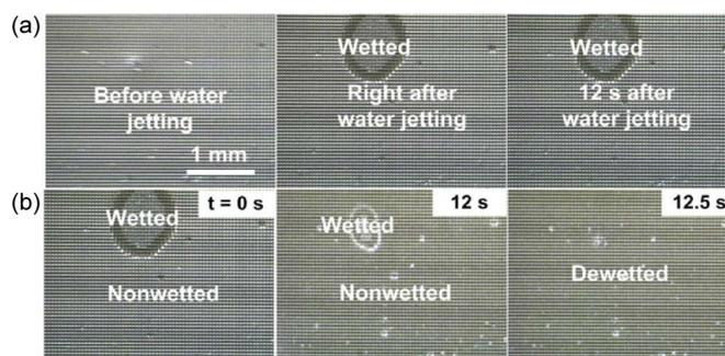
Fig. 7. Hierarchical surface resists against wetting propagation when locally wetted, rendering dewetting easier. (a) For the testing (microposts:  $50\text{-}\mu\text{m}$  pitch and 95% gas fraction), the local wetting was induced by jetting water from a syringe in water. The wetted area remained unchanged over time, as the SHPo bottom surface confined the wetted area from spreading. (b) When the electrolysis was initiated ( $t = 0\ \text{s}$ ), the small wetted area was subsequently dewetted.
