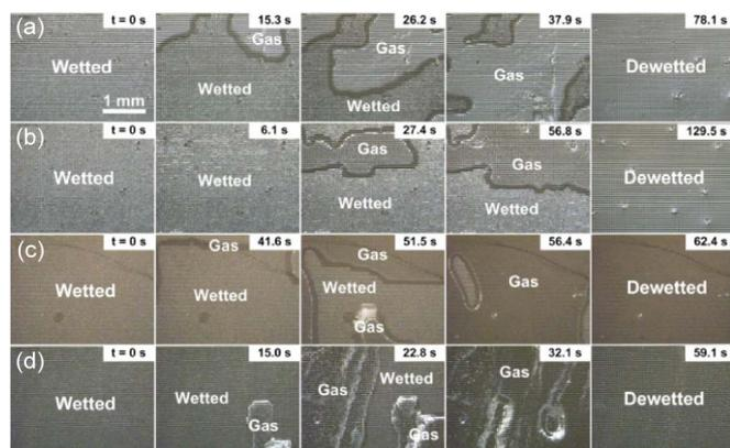
Fig. 5. Dewetting by electrolysis of microposts with a pitch of  $50\ \mu\text{m}$  and gas fractions of (a) 85%, (b) 90%, (c) 95%, and (d) 98%.
