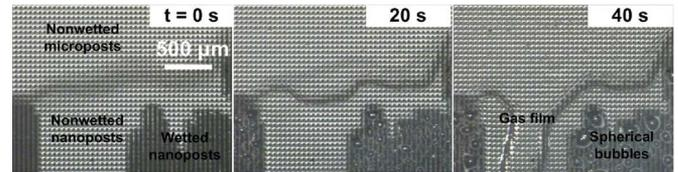
Fig. 9. Gas generation by electrolysis when some of the nanoposts are wetted (by an intentional liquid pressure of 700 kPa above ambient, i.e., 1.7 atm). While a gas film was formed on nonwetted nanoposts, spherical bubbles were formed on the wetted nanoposts.
