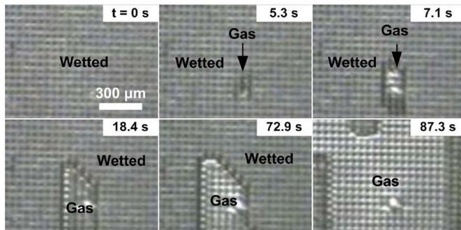
Fig. 4. Formation of a gas layer by electrolysis (microposts: 50- $\mu\text{m}$  pitch and 85% gas fraction). Dewetting began with the nucleation of a gas (5.3 s), followed by the propagation of gas film into the surrounding area.
