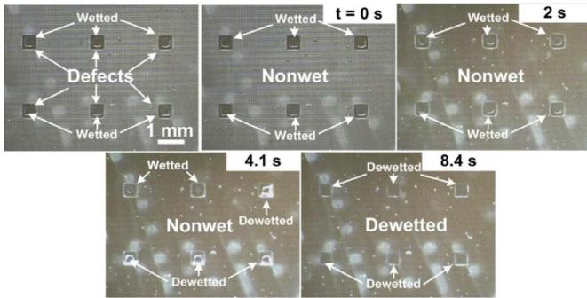
Fig. 8. Dewetting in the presence of defects (microposts: 50- $\mu\text{m}$  pitch and 85% gas fraction). The wetted areas were confined to the defected areas due to the SHPo nature of the nanostructured bottom surface and did not spread to the surrounding area over time. The second image was taken 5 s after the first image, and there was no noticeable change in the wetted area. When the voltage was applied ( $t = 0$  s), the wetted area was easily dewetted by electrolysis.
