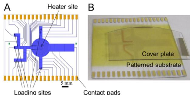
Figure 1: Digital micro-chemical synthesis chip. (A) Design of patterned electrode layer. (B) Photograph of assembled EWOD chip with cover plate and patterned substrate separated by spacers.
