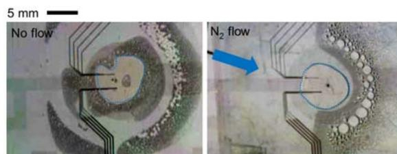
Figure 3: To facilitate removal of solvent vapor during evaporation steps, an inert gas is blown into the space between the parallel plates of the EWOD chip through a needle or vacuumed out through holes in a plate. (Left) Without gas flow, condensation occurs all around the heater site close to the evaporating droplet (blue outline) and can recondense in the droplet. (Right) With gas flow, the evaporated vapor is removed more effectively and evaporation is accelerated.
