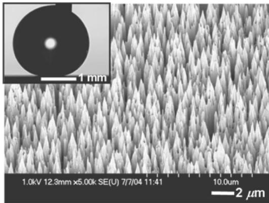
FIG. 2. SEM image of a nanoturf surface made by the black silicon method [24]. The inset shows the apparent contact angle of water droplet (i.e.,  $\sim 180^\circ$ ) on the nanoturf surface after the hydrophobic coating with Teflon.
