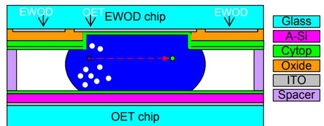
**Fig. 1:** Cross-section of device integrating EWOD and OET. Top glass substrate has EWOD electrodes except central electrode used for OET. Bottom glass substrate contains amorphous silicon for photoconductivity. Oxide and Cytop<sup>®</sup> are patterned on EWOD chip, and only a thin hydrophobic layer covers the OET region.
