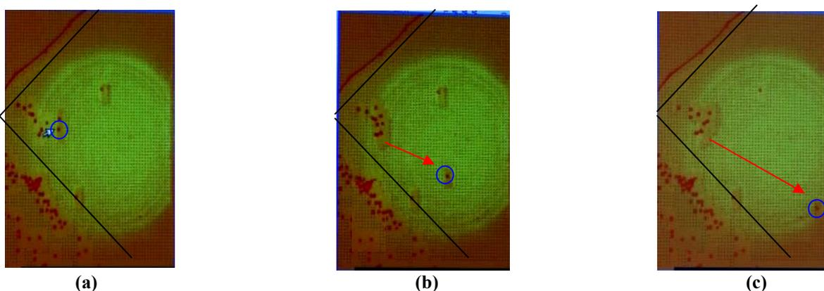
**Fig. 6:** Individual particle control by OET. (a) Specific particle (circled) is chosen by clicking the mouse, triggering the optical pattern to produce rightward movement of that particle. (b, c) chosen particle is moved away from the rest, as indicated by the arrow. Edges of OET electrode were added in figures for clarity.
