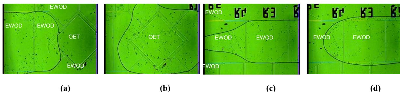
**Fig. 4:** Droplet manipulation by EWOD. (a, b) EWOD operations of bringing droplet with beads into OET region; (c, d) EWOD cuts droplet out of OET region as in Fig. 2(c). The dielectric pattern inside the OET electrode (rotated square) marks active OET region. Surrounding EWOD electrodes are used to move droplets into, out of and around OET region.
