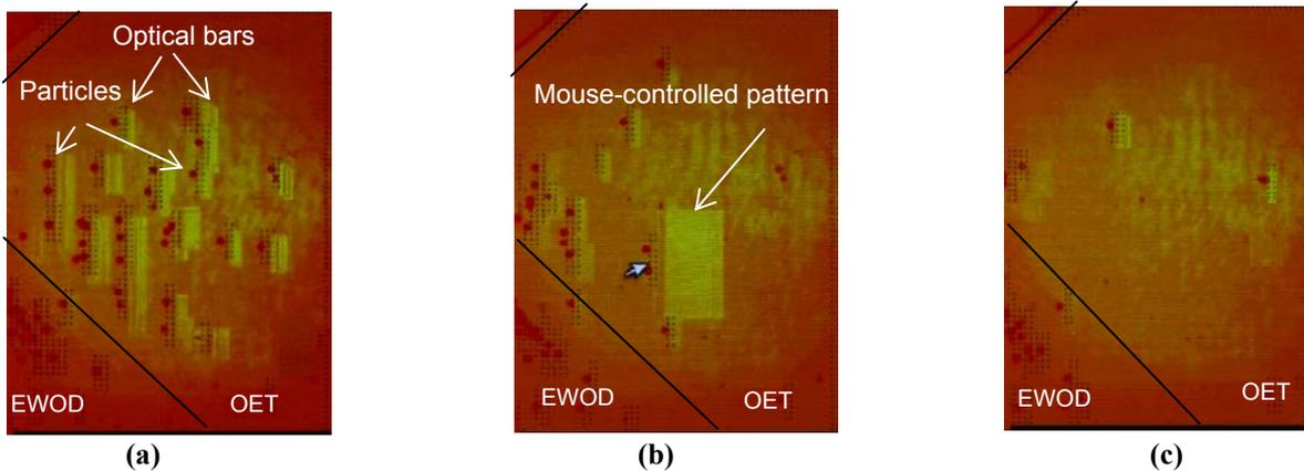
**Fig. 5:** Particles swept by OET. (a) Each particle (dark dot) is pushed to left by an optical bar pattern next to it. (b) Optical patterns, e.g. bar controlled by mouse (or keyboard) can also be used to sweep. (c) Nearly all particles in the OET region have been swept to the left (most are out of view). Edges of OET electrode were added in figures for clarity.
